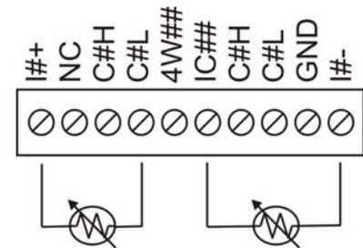
*Two-wire, two-sensor measurement configuration*
