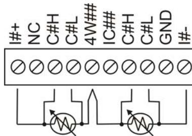
Four-wire, two-sensor measurement configuration
