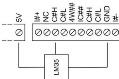
Semiconductor sensor measurement configuration
