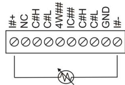
*Two-wire, single-sensor measurement configuration*
