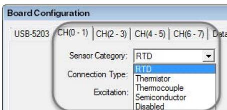
Channel pair tabs and the Sensor Category list on the Board Configuration dialog box in InstaCal.
