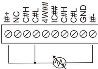
Three-wire, single-sensor measurement configuration
