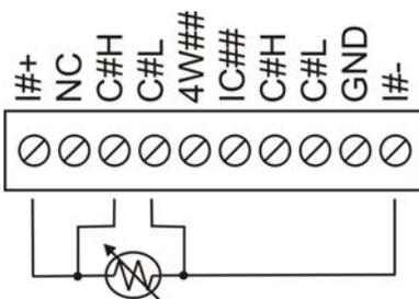
Four-wire, single-sensor measurement configurations
