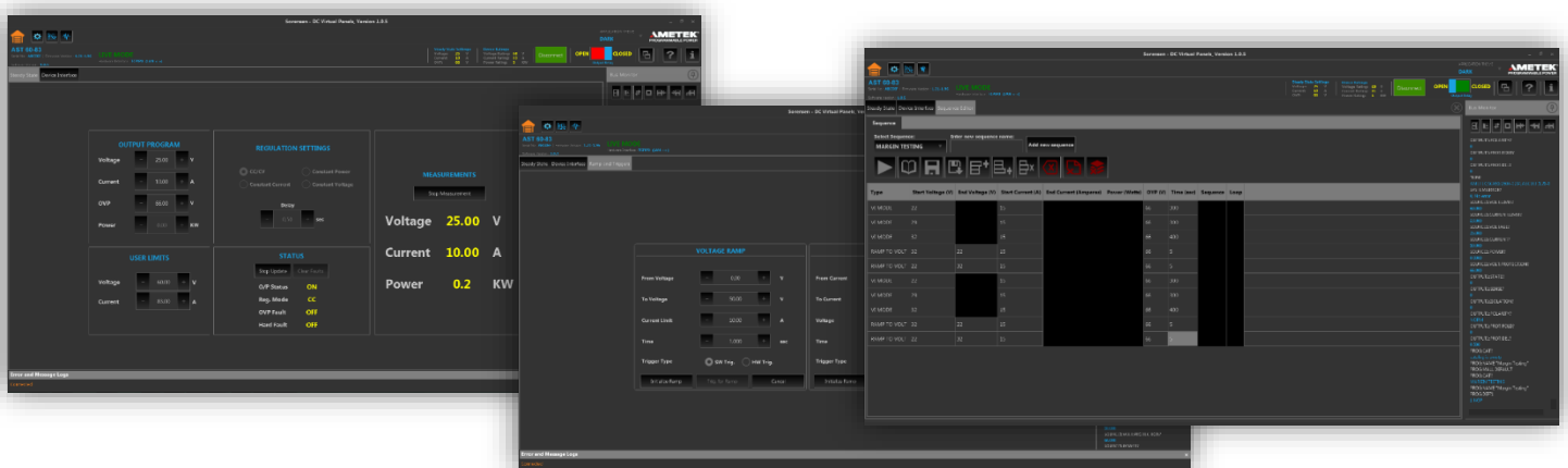
Virtual Panels “main status,” “sequencing” and “output ramp” screens are shown.
